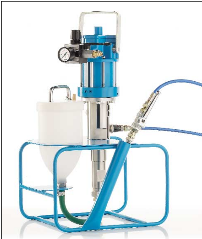
The WIWA Inject HD 1 is equipped with a feed funnel for approx. 1.5 liters (3 pints) of resin and an injection lance.
