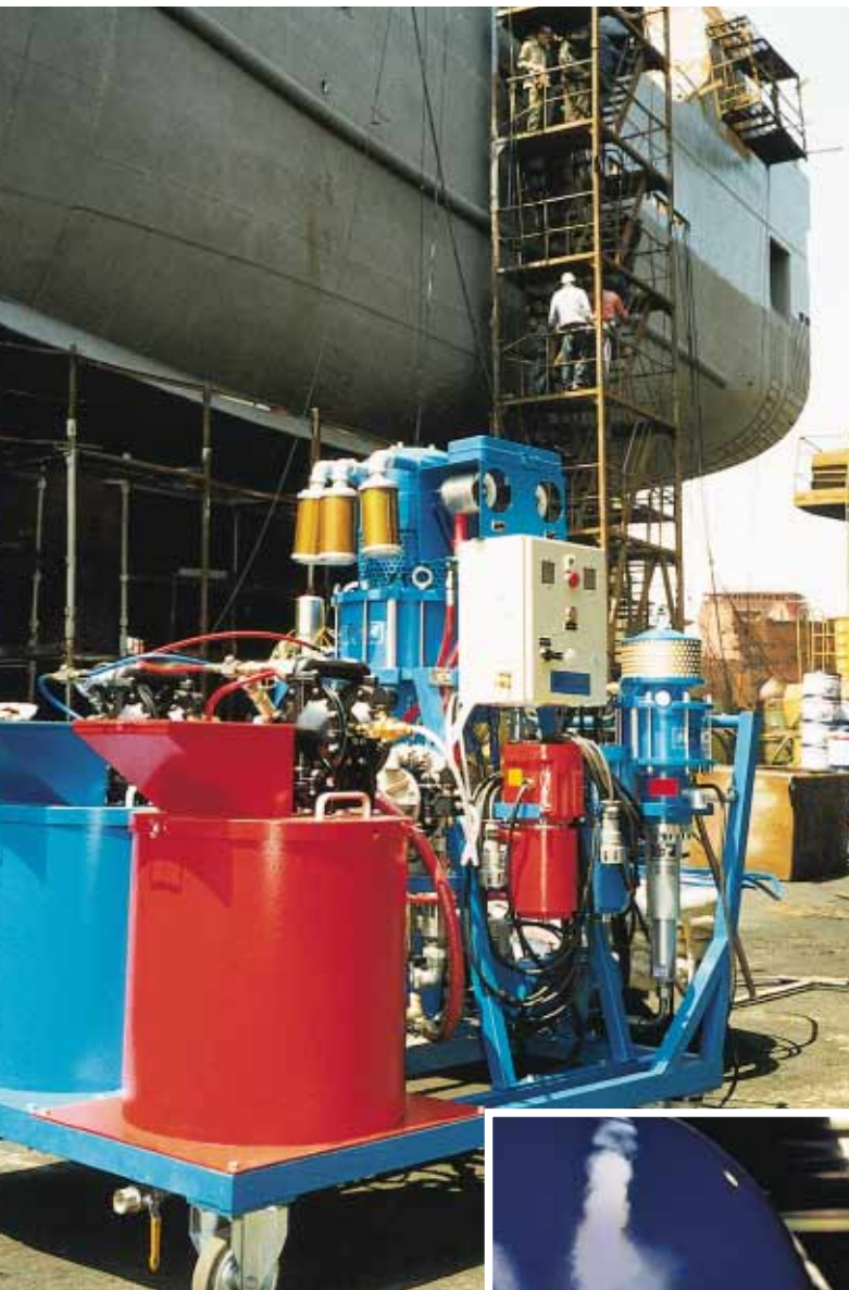
Here, an icebreaker is being sprayed with a special coating material (potlife: 5 minutes, spraying temperature: 55°C) using a WIWA DUOMIX 333 with heated hoses.
