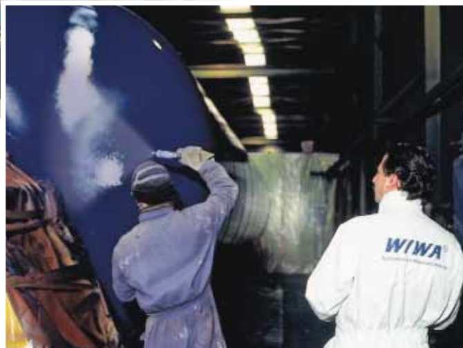
Here, an icebreaker is being sprayed with a special coating material (potlife: 5 minutes, spraying temperature: 55°C) using a WIWA DUOMIX 333 with heated hoses.
