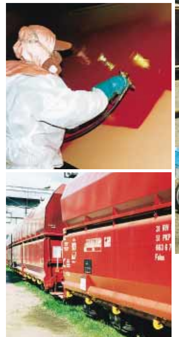
A railcar for transporting food is being coated with a solvent-free, thick polyurethane coating using a WIWA DUOMIX 333 (solids: 92,5%, potlife: 5 minutes, spraying temperature: 60°C).
