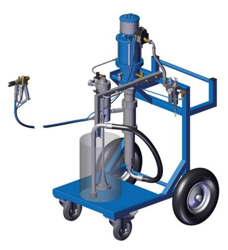
Foundry washes create a sealed surface between the sand and metal necessary to allow the release of the piece from the form after casting. Black wash is applied through spraying in the fluid state using a WIWA Low Pressure Pump DA 10:1.
