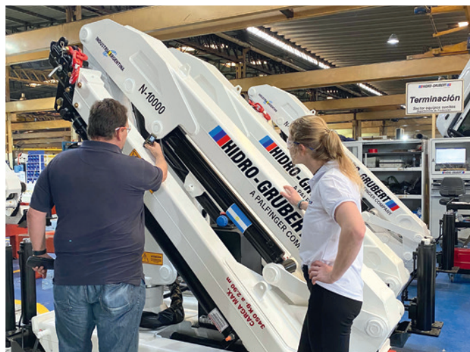
Angelika Zeilinger and a service specialist from Mankiewicz check the layer thickness at the new paint shop in Argentina.
