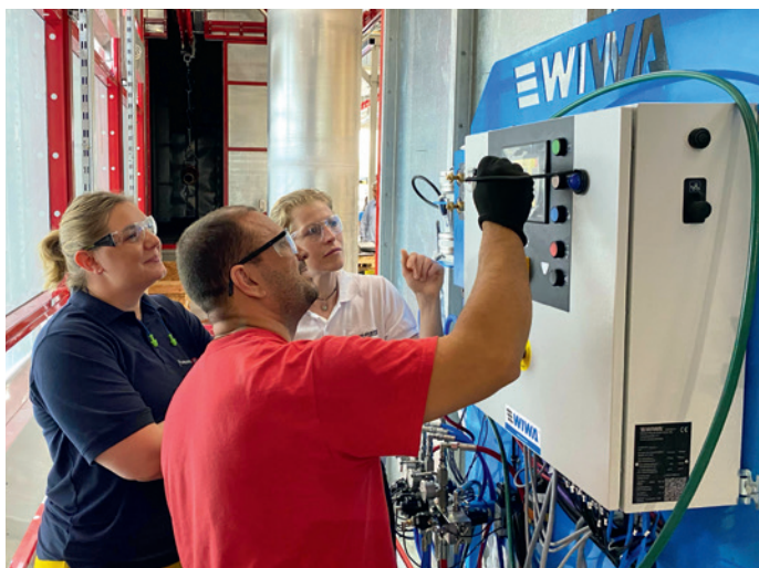
Joint mixing and application parameter settings at the newly installed systems from WIWA.
