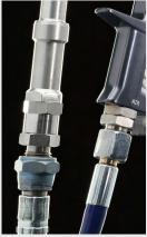
Ball bearing swivel joint at the paint connection. Swivel joint at the air connection.
