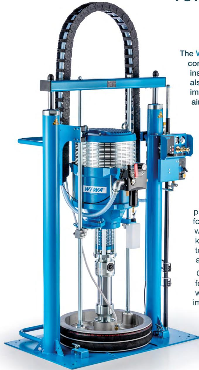
The **WIWA VULKAN GX** extrusion pumps for conveying, dosing and applying adhesives, insulating materials and sealing materials now also rely on the new WIWA GX air motor. This impresses with a full metal housing, optimized air distribution during operation to minimize icing during continuous operation and reduced noise.
