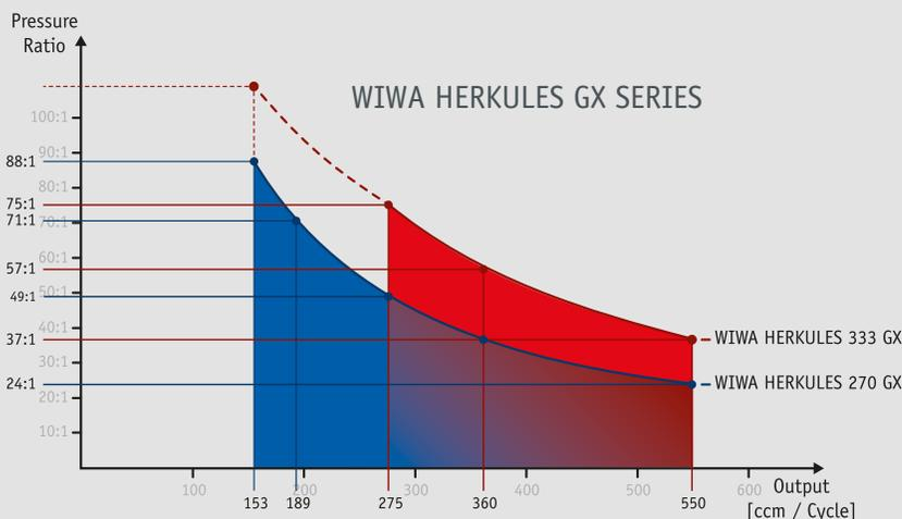
The graph shows the different output values at the given pressure ratios for each pump.
