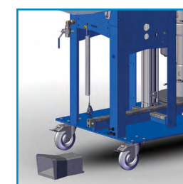
Start-stop function via foot control
