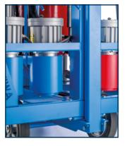
Electronically controllable material flow heaters
