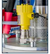
Radar sensors for level control
