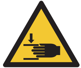
Fig. 1: Warning about the risk of crushing
